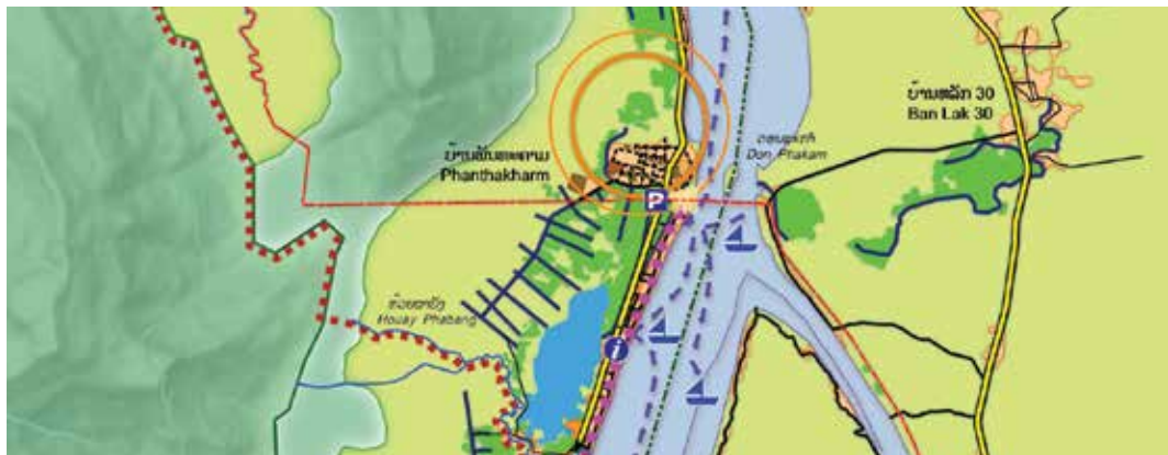
Fig.120: Extract from the Master Plan where one can see the development pole at the north entrance of the site, roads, river links, the irrigation system and irrigated rice fields, as well as the lake wetlands.
